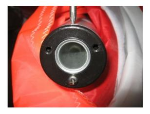
• Using a pair of needle-nose pliers pushed into the two holes in the head of the cam, rotate the cam to the degree desired. In the example described above, the cam will have to be rotated 5 mm clockwise.
